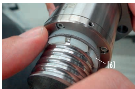
Fig. 4.15 Removing the finger wiper
