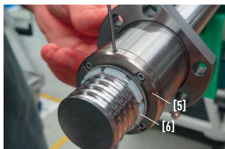
Fig. 4.14 Loosening the grub screws
