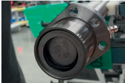
Fig. 4.10 Removing the metal ring
