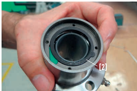
Fig. 4.12 NBR wiper [2] and support ring [1]
