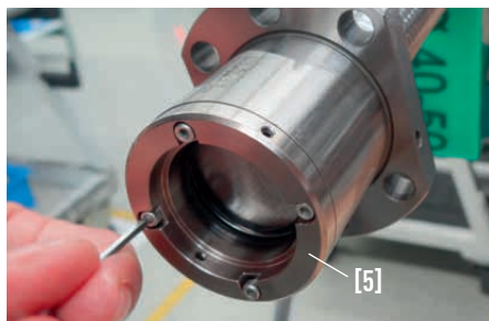
Fig. 4.16 Unscrewing the wiper housing
