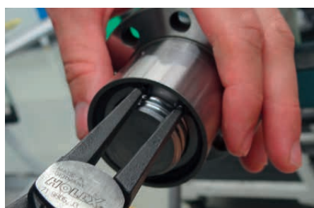
Fig. 4.9 Removing the circlip
